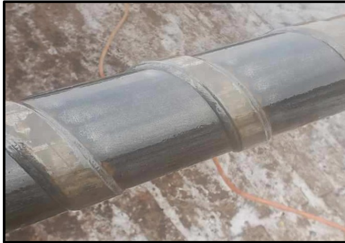
Wear exhibited by of the Spiralbanding after 13 wells drilled
