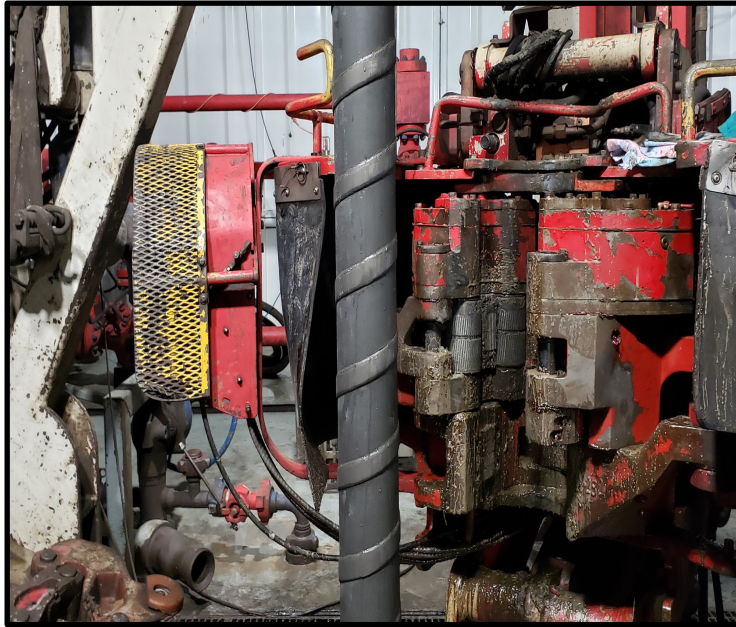
Spiralbanding condition after 4 wells drilled
