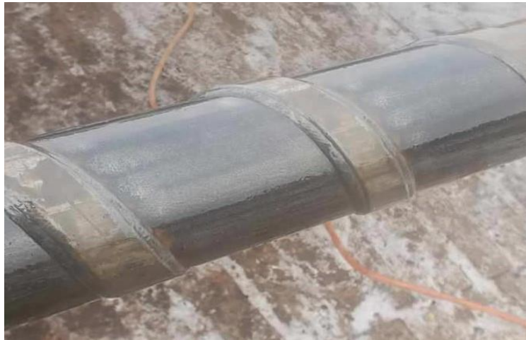
40% of the Spiralbanding remaining after 13 wells drilled
